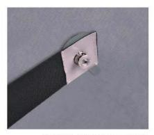
Fixation inside the vehicle with heavy-duty suction pads: strong assembly on any vehicle, even if fitted with cab screens
