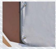
Hanging on passenger side using Tenax® self-locking fasteners
